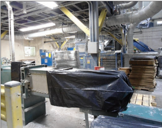
A plastic bag collects paper dust which will be mixed with paper bales and recycled.
