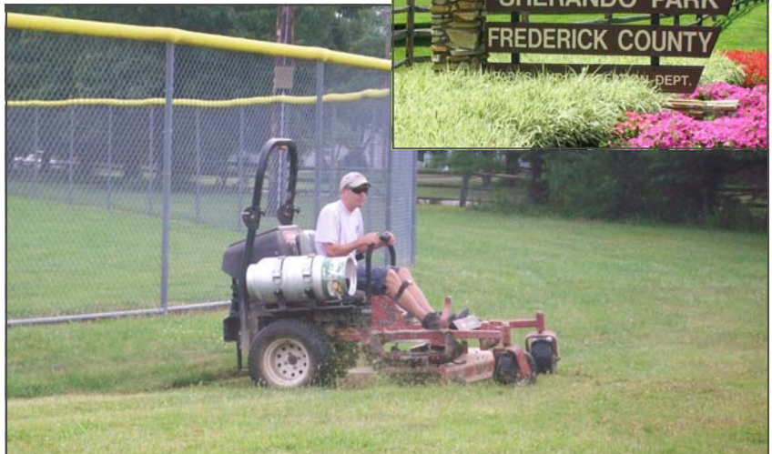
Parks staff using a mower converted to propane at Sherando Park.
