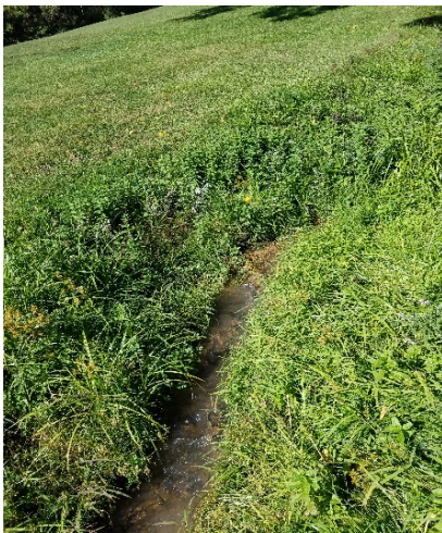
(Leak emerging from the ground)
